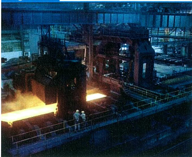
Mesta 140-inch 4-high and vertical edging mill.
